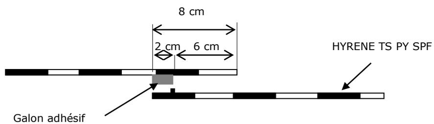
**Figure 8 – Recouvrement HYRENE TS PY SPF**
