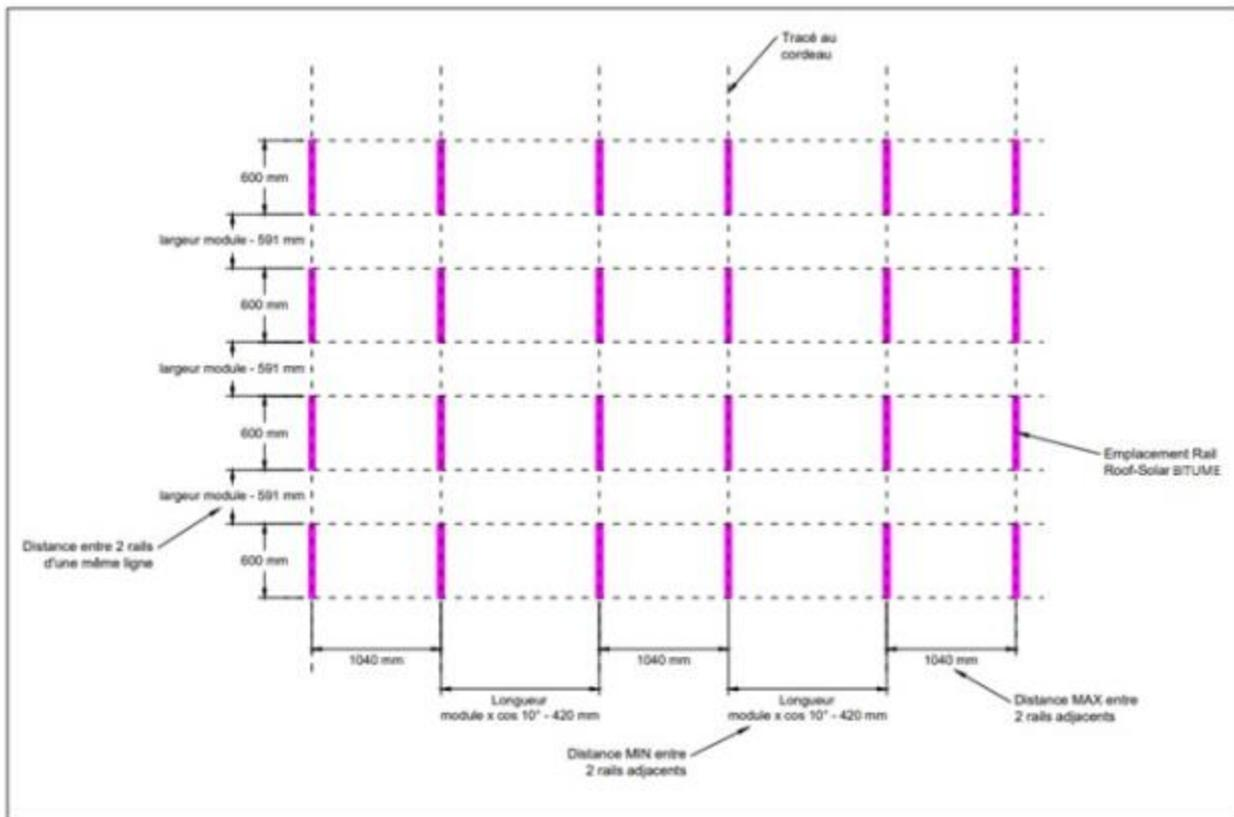
**Figure 29 (suite) – Traçage des rails – configuration simple shed**
