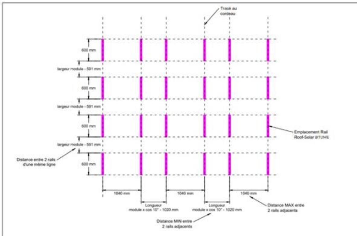
**Figure 29 (suite) – Traçage des rails – configuration double shed**
