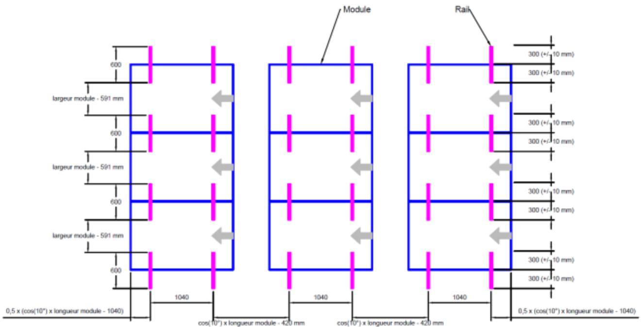
Figure 35 - Implantation des rails / modules simple shed
